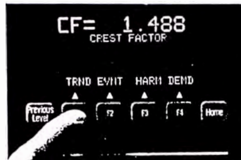
Operator About to Access the Trend Analysis Screens
