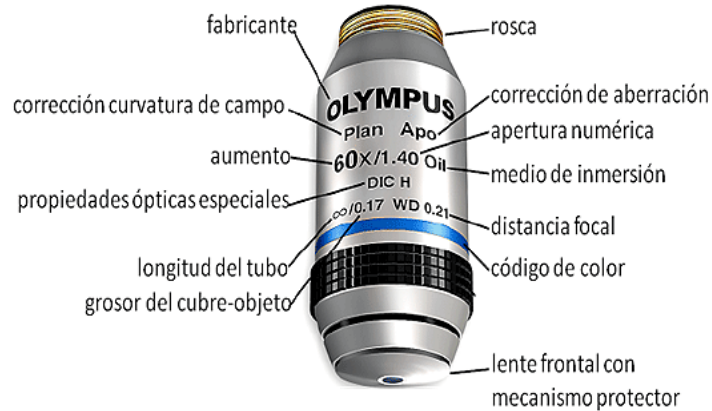
Figura 17: Nomenclatura de la Lente (Fuente: Edmund Optics, Understanding Microscope and Objectives. )
