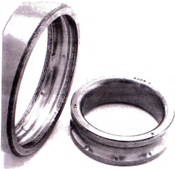
Figure 23 — Overloading during mounting
