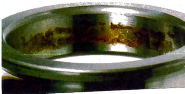
Figure 14 — Fretting corrosion in inner ring bore
