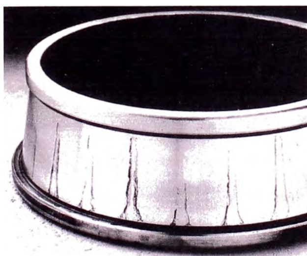
Figure 13 — Contact corrosion on a bearing raceway
