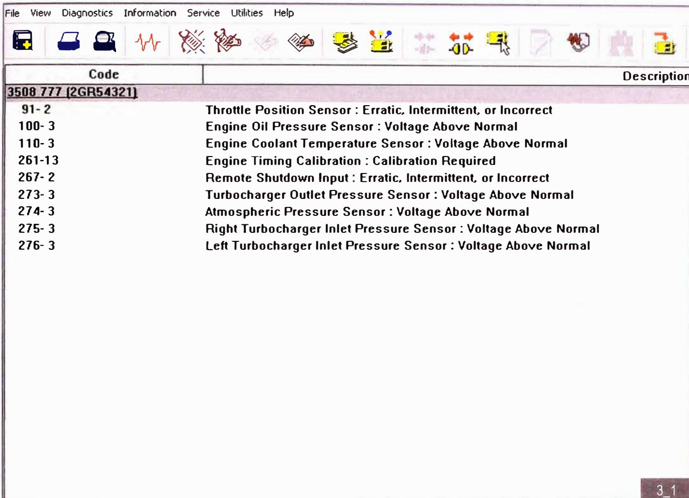
The screenshot shows a diagnostic software window with a toolbar at the top containing icons for File, View, Diagnostics, Information, Service, Utilities, and Help. Below the toolbar is a list of fault codes (FMs) for a Caterpillar engine. The list includes:
