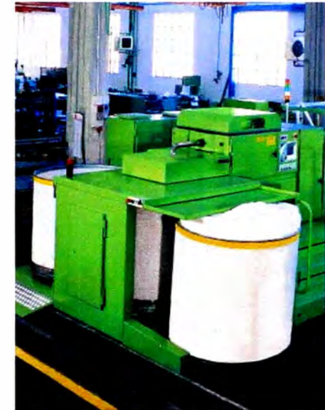
Cambio trasversale dei vasi addossato (V11T) Rectilinear can delivery positioned against the machine (V11T)
