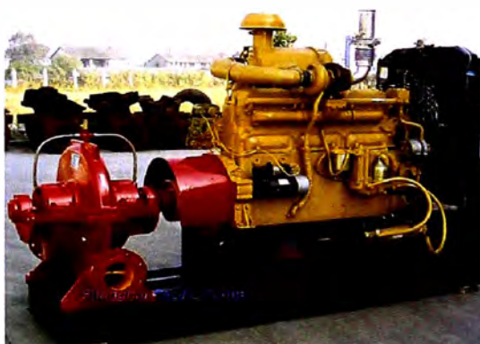
Figura 2-12: Motor Diesel-Bomba Contraincendios
