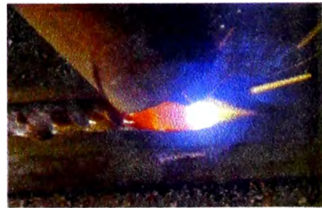
FIGURE 10-20 Forehand welding or push angle. Courtesy of Larry Jeffus
