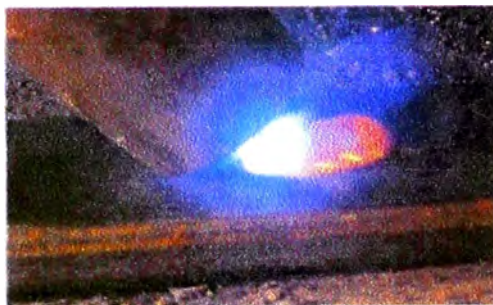
FIGURE 10-19 Backhand welding or drag angle. Courtesy of Larry Jeffus
