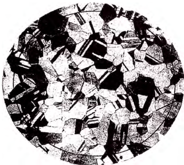
FIG. 3 Example of Twin Grains (Contrast Etch) from Plate III. Grain Size 0.090 mm at 75x
