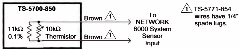
Figure 2 TS-5700-850 Series Sensor Connections.
