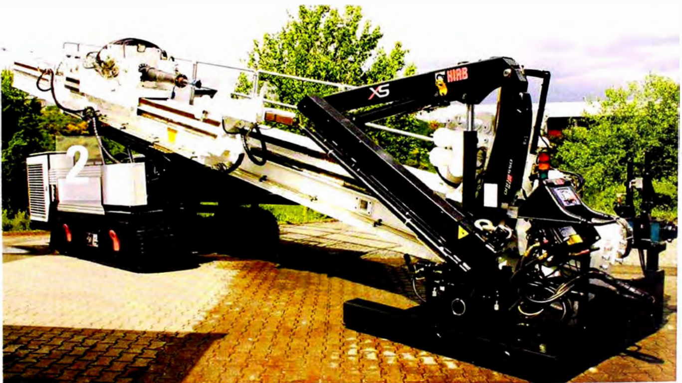
Bore unit with integrated hydraulic powerpack
