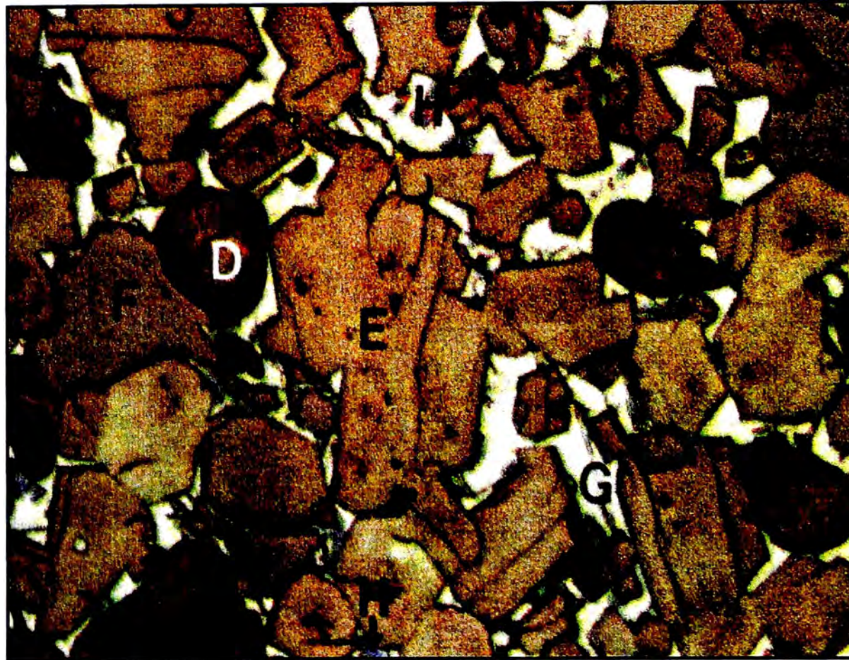
Fig. 10 E: Alita C_3S ; D: Belita C_2S ; F: Poro; H: Aluminita C_3S G: Ferrita C_4AF .
