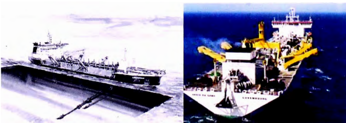
Figura 2.03. Dragas Trailing Suction Hopper Dredger.
