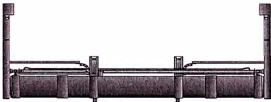
DCE 70 attachment with twistlocks, length adjustments 20-40'. Attachment with hook connection, side-shift \pm 140 mm. Mechanical levelling on each side.
