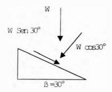
Pot tornillo = FxV = Wpeso x  $\mu$  x Sen  $\beta$  x w x r = 400 Kf x 0.5x1x200  $\underline{rev}$  x 0.075 m 2 60  $\underline{seg}$
