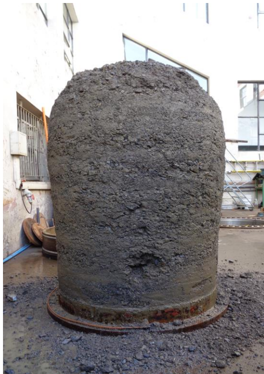
Foto 6: Probeta 100x180 cm ensayada a 20.0 kg/cm 2
