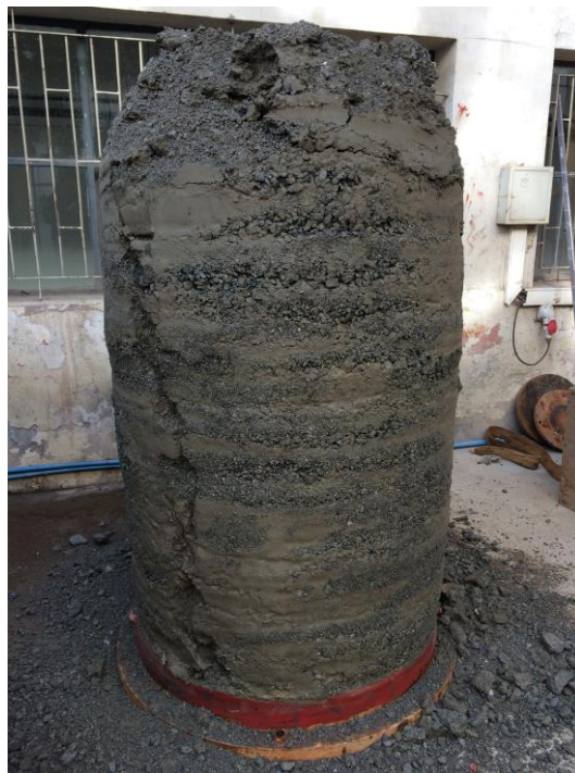
Foto 5: Probeta 100x180 cm ensayada a 10.0 kg/cm 2
