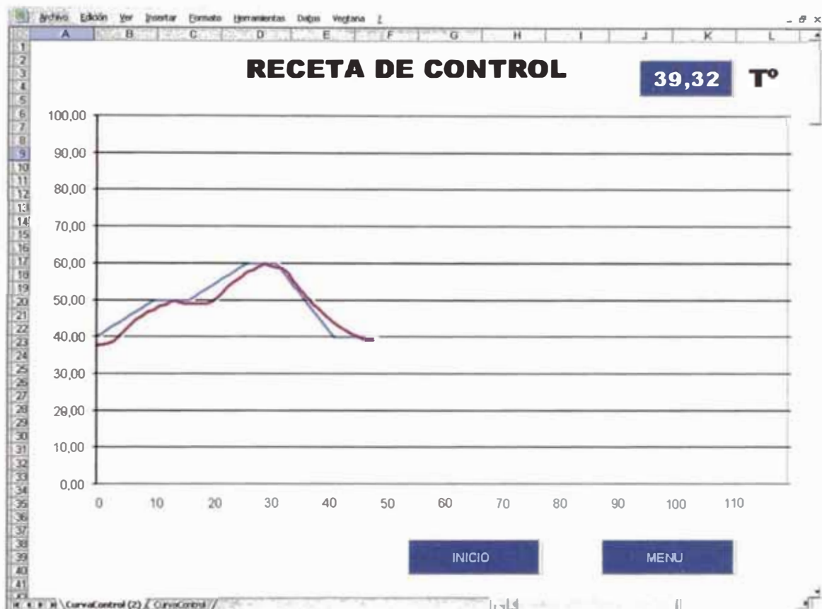
Figura 72: Control Temperatura Setpoint Variable
