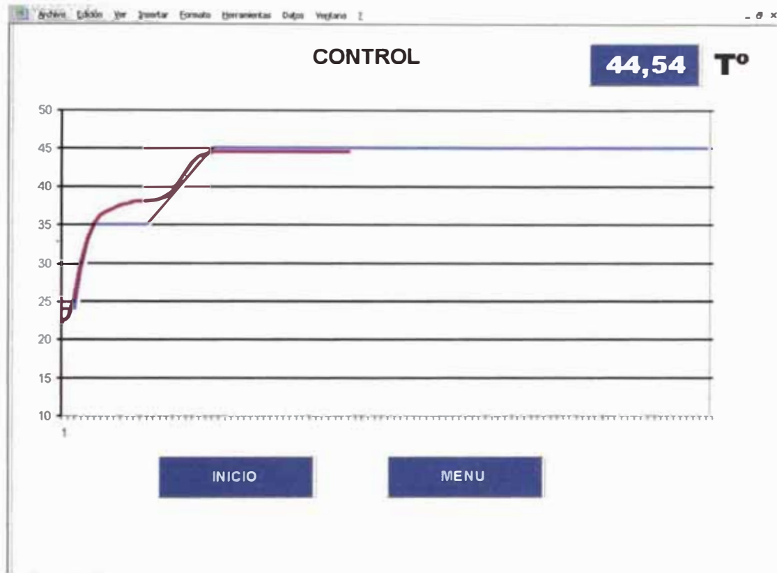
Figura 71: Control Temperatura Setpoint Variable
