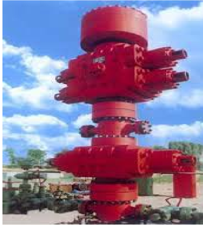
Blow out preventor (BOP)
