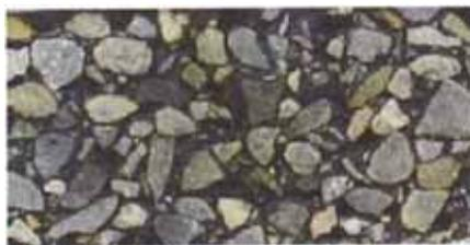
Figura 4.1(a) Stone Mastic Asphalt
