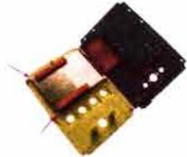
② Fold the main board over while keeping LCD in place.
