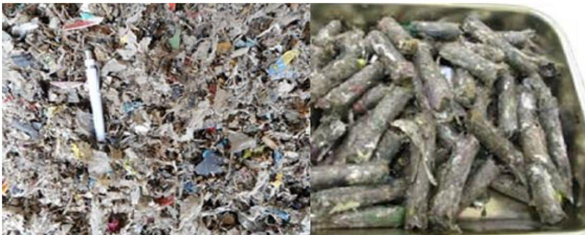
*Nota.* (I) CSR sin compactación. De “Design, quality and quality assurance of solid recovered fuels for the substitution of fossil feedstock in the cement industry – Update 2019”, de Sarc et al., 2019, *Waste Management & Research*, 37(9), p. 889 (doi: 10.1177/0734242x19862600). (D) CSR compactado. De “Characterization of Korean solid recovered fuels (SRFs): an analysis and comparison of SRFs”, de Choi et al., 2012, *Waste Management & Research*, 30(4), p. 443 (doi: 10.1177/0734242x12441239)
