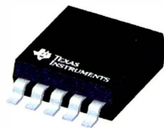
Figura 4.34. 16-bit, 860-SPS, 4-channel, delta-sigma ADC with PGA, oscillator, VREF, comparator and I 2 C [128].
