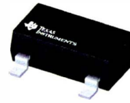
Figura 4.33. 2.048-V, 30-ppm/°C drift, 3.9- \mu A, 3-pin SOT-23, 3-pin SC70, 8-pin UQFN voltage reference.
