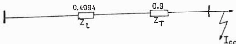
$$I_{cc10kv} = \frac{10,000}{3 \times 9.494} = 607.80 \text{ AMP}$$
