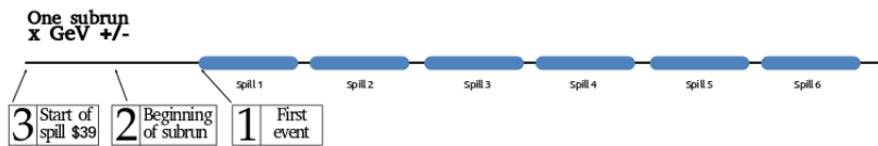
(a) Diagram of the three points of reference that can be used in the calculation of the time profile .
