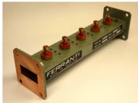
(b) Five-resonator triple-post waveguide band-pass filter made by Ferranti. Source Wikipedia CC1.0.
