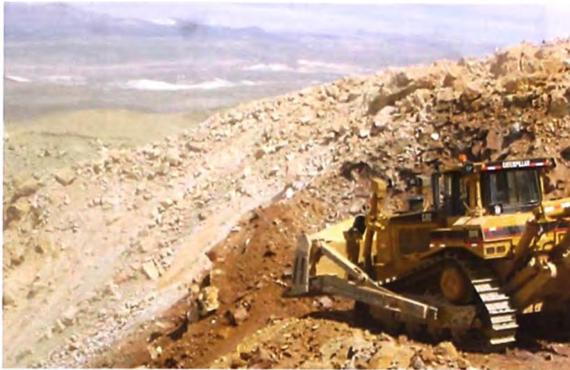
**Fig18 Tractor Oruga D8R**
