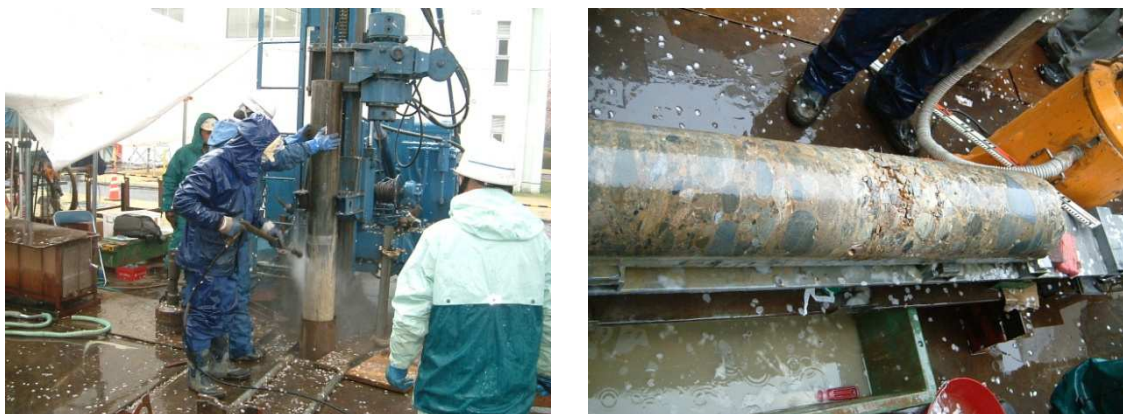
Fotos 3.6 y 3.7: Método reciente de muestreo de gravas utilizando polímeros. Undrained Strength of Gravelly Soil During Earthquakes-Takaji Kokusho – Professor of Chuo Univeristy
