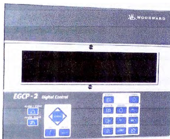
Figura 2.6 Controlador EGCP-2, panel frontal
