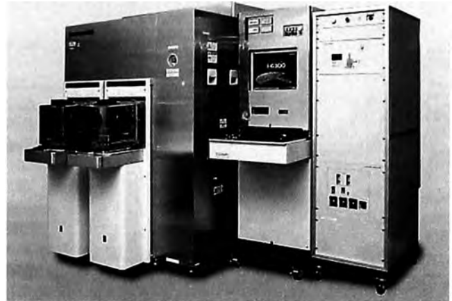
High-sensitivity high-speed SEM visual inspection system: I-6300
